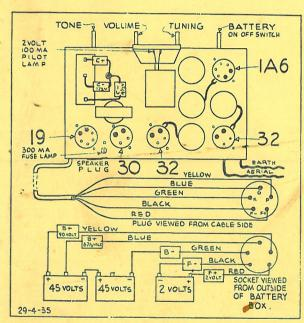
This is a new model designed to give extreme economy of battery consumption with reasonable amount of sensitivity and audio output. This model has been held in the Laboratory longer than was expected, to make exhaustive tests, not only on the economy of battery drain, but to ascertain what performance could be expected from such a model under various conditions.
